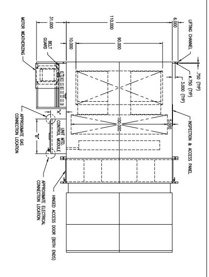
BLOWER/BURNER HEAT SECTION V-BANK FILTER SECTION INLET DAMPER FRESH AIR HOOD (SHIPPED BROKEN DOWN FIELD ASSEMBLY REQ.)
